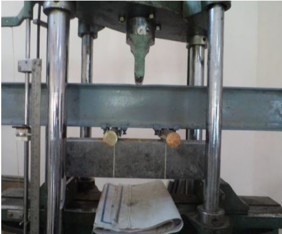
Fig. 3.4: Specimen loading for flexural strength test
