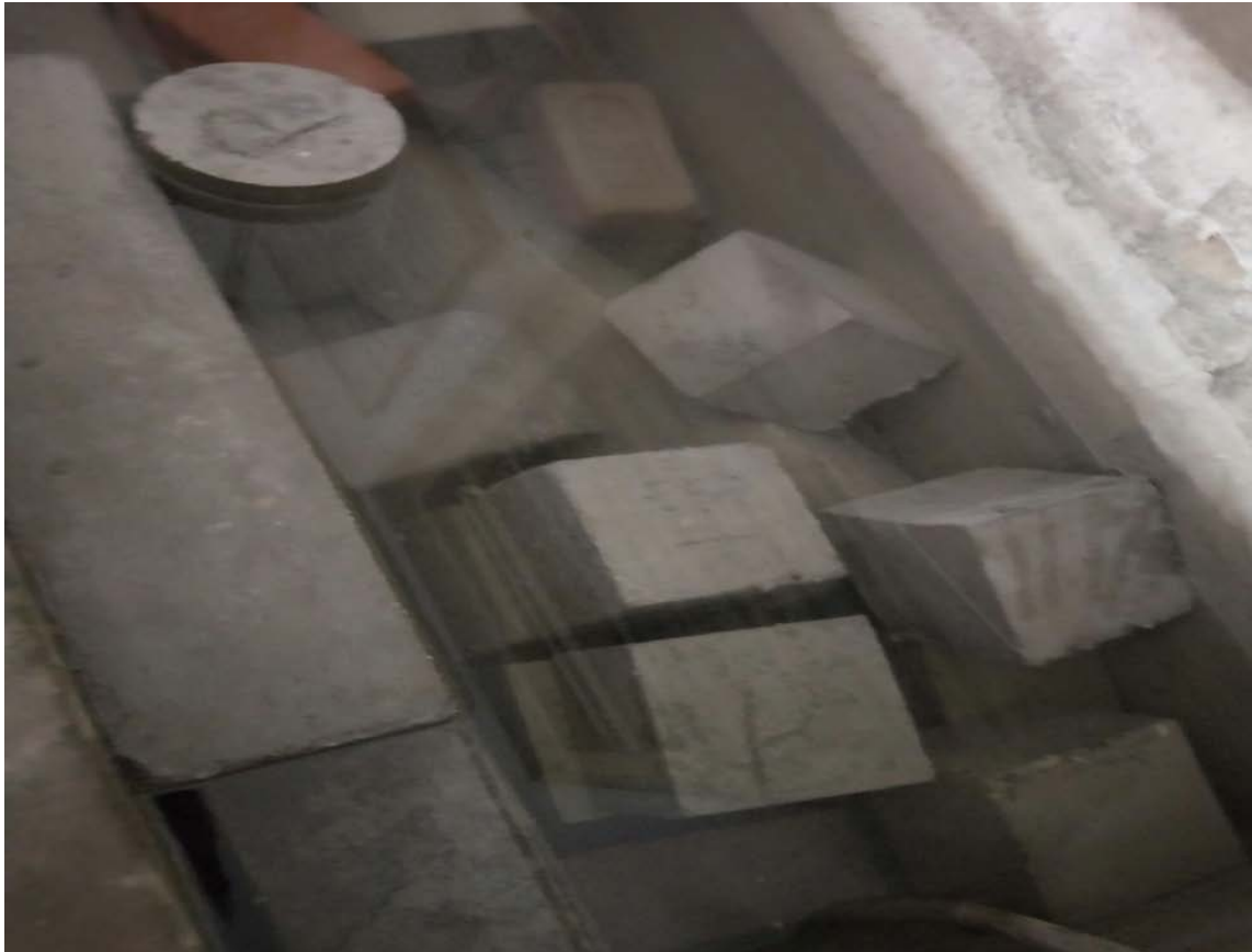
Fig. 3.2: Curing of cubes, beams and cylinders
