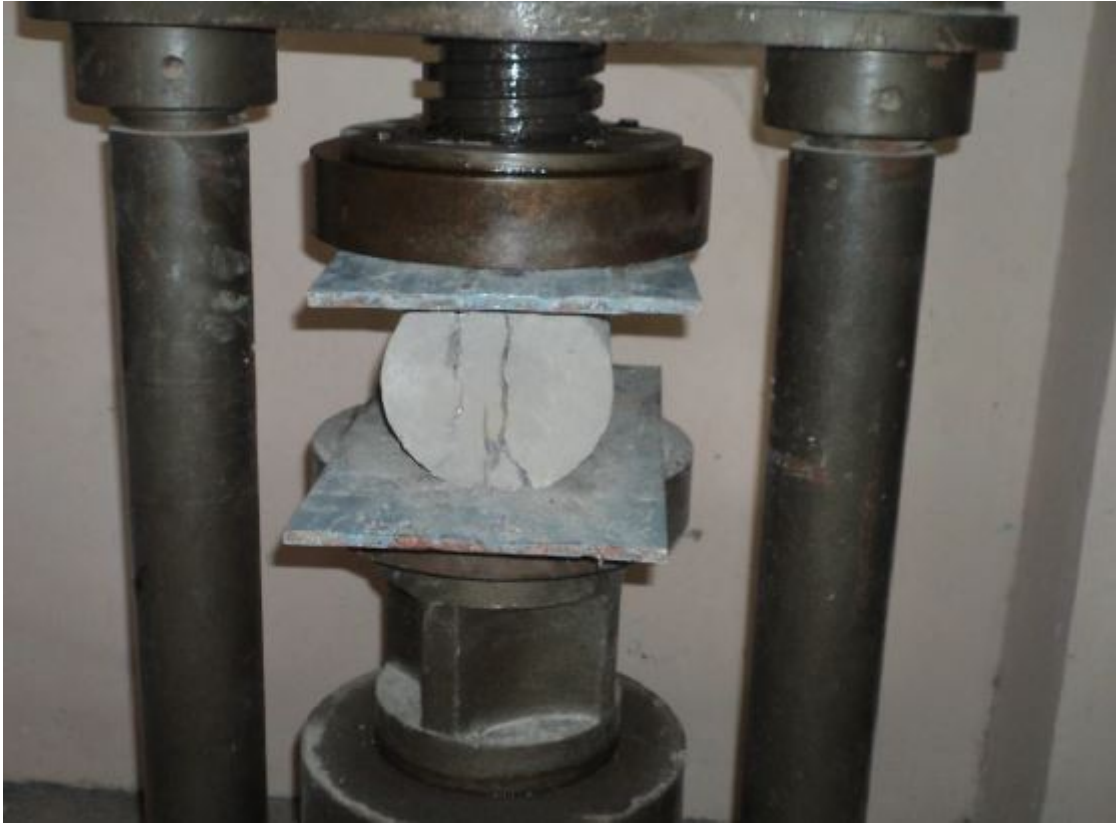
Fig. 3.5: Specimen loading for split tensile strength test
