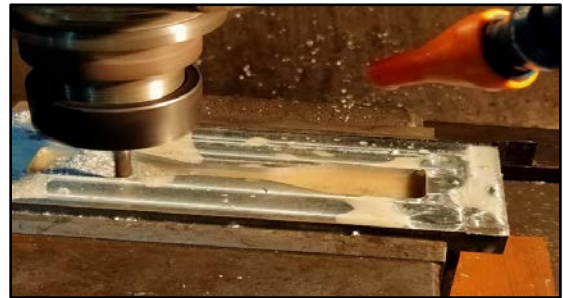
Figure 14. Visualization of the die manufacturing on the vertical milling machining
