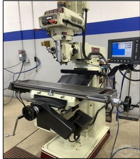
Figure 13. CNC vertical milling machine used for die and punch manufacturing
