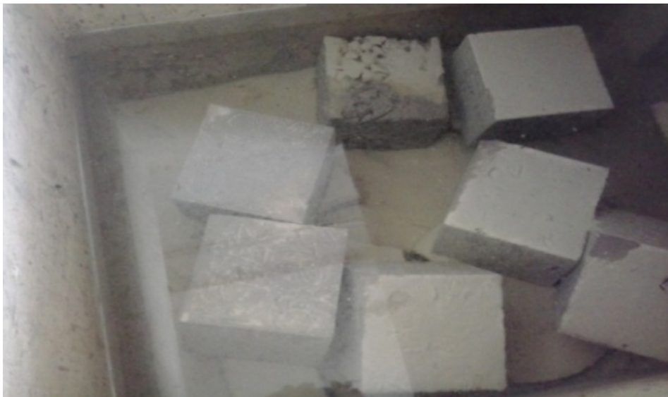
Fig. 3.8: Curing of cubes and Beams
