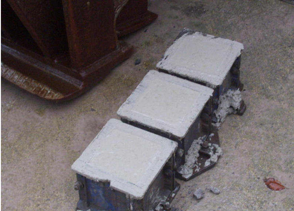
Fig. 3.7: Casting of Cubes
